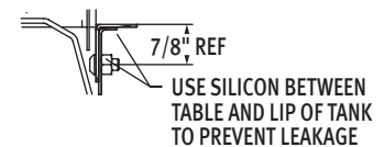
Sectional View Showing Table Connections
