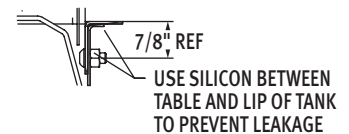
Sectional View Showing Table Connections
