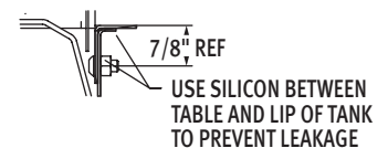
Sectional View Showing Table Connections
