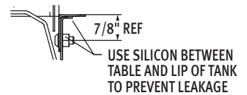
Sectional View Showing Table Connections
