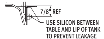
Sectional View Showing Table Connections
